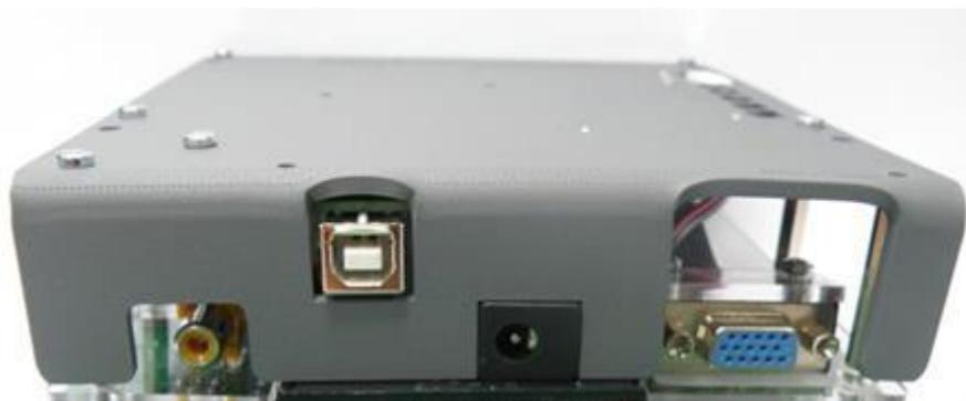
Mounting the FMC is quite easy where you can either mount it using the small mounting holes on the front panel – this however specifies that the panel where the FMC is to be mounted in must only be a few millimeters thick otherwise this cannot be done properly. Another way to mount the FMC is to use the edge holes on the back casing where you then have the ability to fasten the FMC to any type of bracket or stand or similar.
