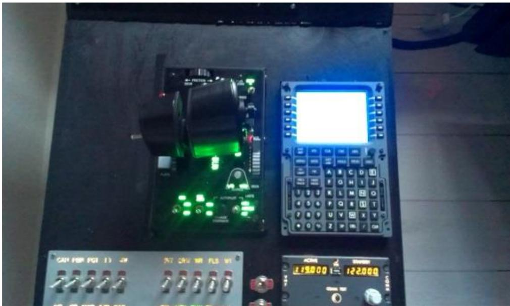
The FMC also features a dimmable backlight function which works perfectly. To control the backlight you simply just use the small rotator/encoder located just above the Execution button and the backlight goes from completely dark (off) to bright. Easy and very realistic which gives the simmer a superb experience when using the FMC for night VFR/IFR – this of course also means that the light in the room where the flight simmer is flightsimming has to be off.
